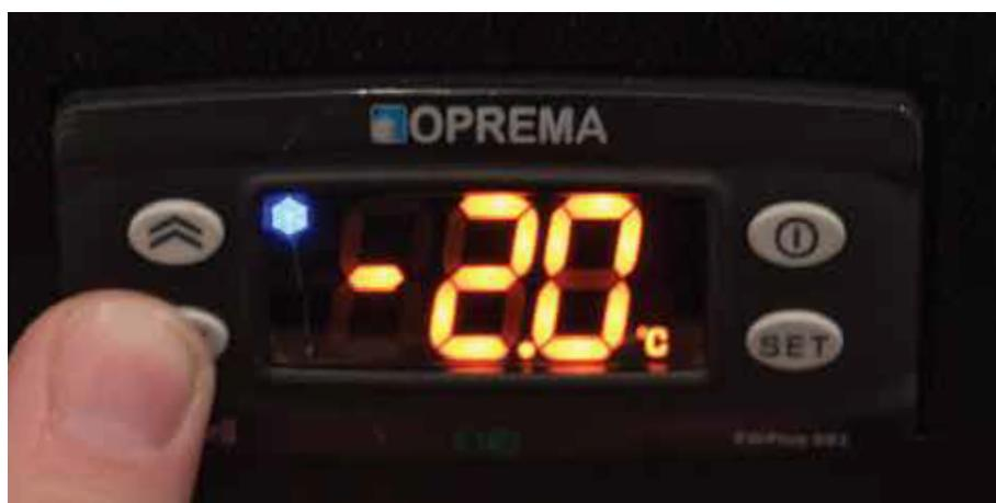
Press Power Button two times to leave the settings menu and return to normal operating mode.
